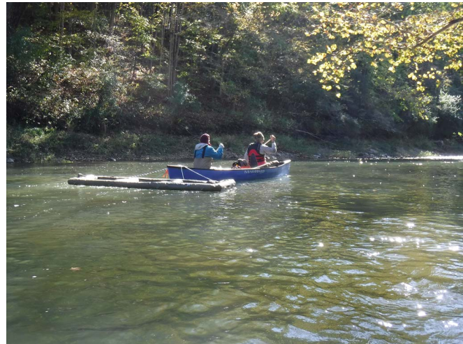
Figure 2. Example of a single-cable inflatable (floating) antenna used to cover large areas ( \sim 1 m) to improve detection of passive integrated transponder tags placed on native freshwater mussels in the Vermilion and Kishwaukee rivers, Illinois. Photo by Alison Stodola.
